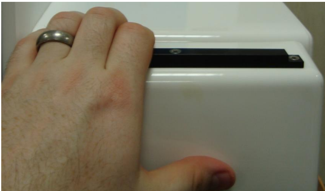
Fig.15 Interlock outer door opening
