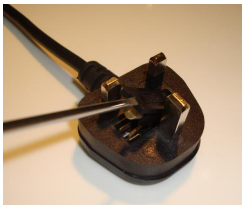
Fig.28 Mains plug fuse removal
