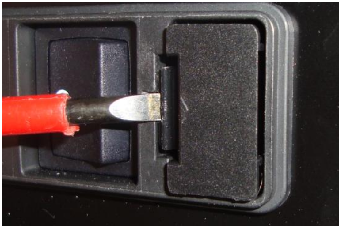
Fig.29 mains fuse holder removal
